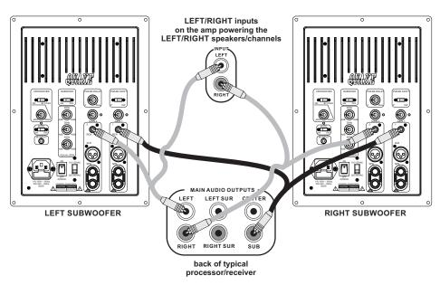
**NOTE:** This same wiring configuration can be duplicated for the XLR inputs. However, we do <u>not</u> recommend mixing input types even though we provide you with three (3) different input types.
