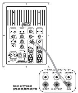
Typically one RCA can feed enough signal to drive the IQ amplifier to its full potential. However, in some cases where the signal is too low for the IQ amp to produce its full output, you may use a "Y" connector to increase the amp's sensitivity.
